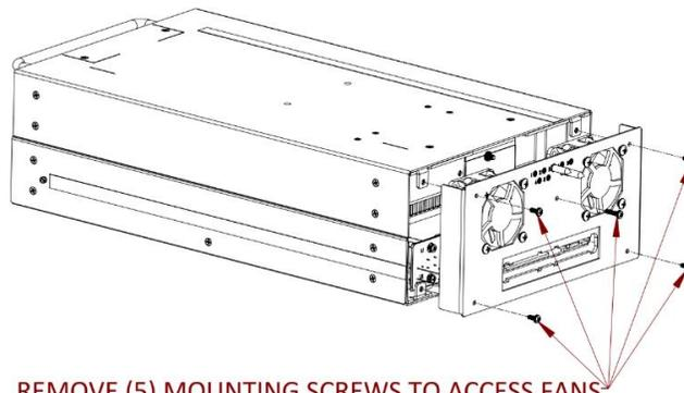
REMOVE (5) MOUNTING SCREWS TO ACCESS FANS
