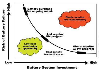
Users can achieve higher battery system reliability by spending more on maintenance and monitoring equipment. But monitoring equipment that is too complex to be of practical use represents both wasted investment and false security. Simpler battery monitoring solutions that are integrated into products already needed at the site, like chargers, can provide useful monitoring function at virtually the same price as conventional chargers, thus delivering excellent return on investment.
