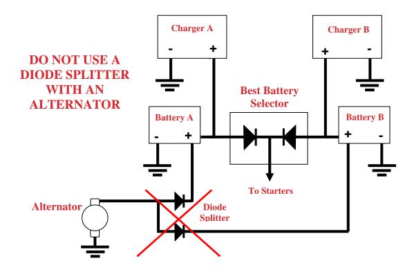
If an alternator is required to be connected into the system, the alternator should be connected directly to the battery it is charging, not connected through a diode. If two alternators are used, Alternator A should be connected directly to Battery A, and Alternator B connected to directly to Battery B, with no diodes or cross connections used.
