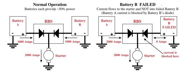
A BBS performs the valuable functions of coupling good batteries, and isolating a failed battery
