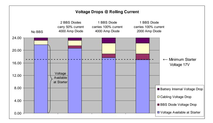
This data shows that minimizing voltage drops in the BBS is critical to reliable engine starting. The installer must minimize cable lengths, use the largest possible wire, parallel two or three times if possible, and insure tight crimps and connections. In order to properly size batteries for an engine starting system with a BBS, the genset package supplier will need to obtain data on engine cranking amps from the engine manufacturer, and BBS diode voltage drops from the BBS manufacturer.
