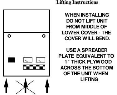
The charger can be mounted either on a wall or in a standard 23" relay rack. Locate the charger in a dry place as close to the battery and load as possible to minimize voltage drop.
