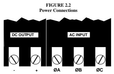
Connection should be made by a qualified installer in accordance with national and local electrical codes. The installer should determine the gauge of wire to be used based on the length of cable run and the ampere requirements of the charger. Size the DC cabling to keep voltage drop in the charging leads as low as possible.
