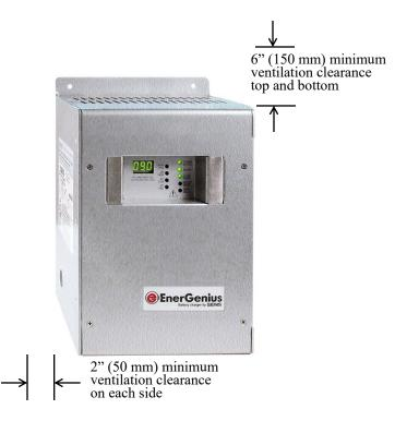
Mount to vertical surface of 3/4" (19 mm) plywood or other material of equal strength and durability, using four mounting screws 1/4" (6 mm) diameter.
