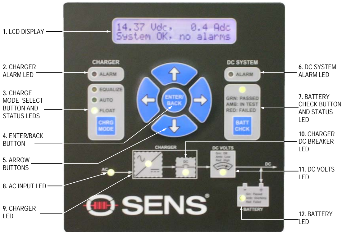
Figure 4: Front Panel User Interface
