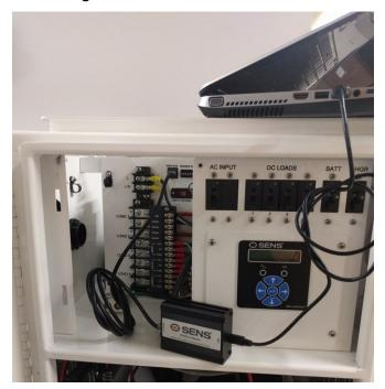
Figure 7 – Standard SENSbus Connection
