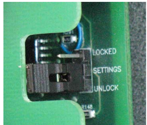
Fig. 7 Front panel jumper UNLOCKED
