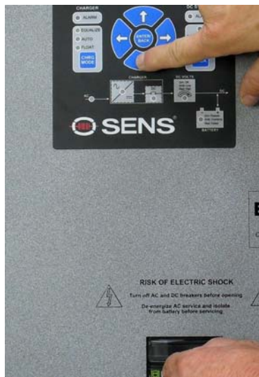
Fig. 12 Starting control processor update
