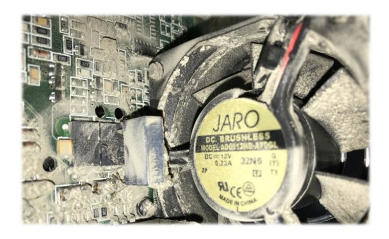
Note dirt caked onto fan blades and layered onto electronic components
