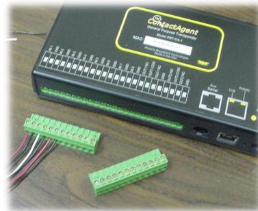
Each interface point consists of a wire clamping receptacle and a clamp screw. The interface is arranged as 8 contact-closure inputs and 2 sets of Form-C (SPDT) relay outputs. 10 common ground points are interspersed among the input and output interface points. See the picture to the left.
