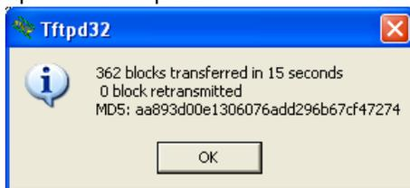
Press **OK** and continue with the next file. The local and remote files names for the 4 **ContactAgent** files are shown in the table below.
