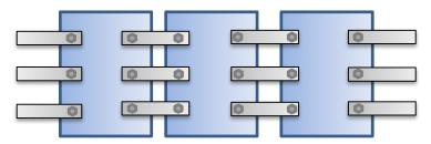
In every case shown, the combination of the jar's internal resistance and its connection resistances forms a "loop" of resistances that gets multiplied by the number of jars in the string. A partial view of the loop resistances in a string of jars is shown below:
